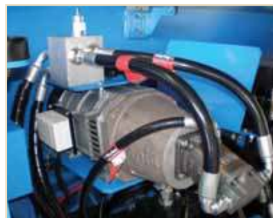
7 KVA HYDRAULIC GENERATOR
